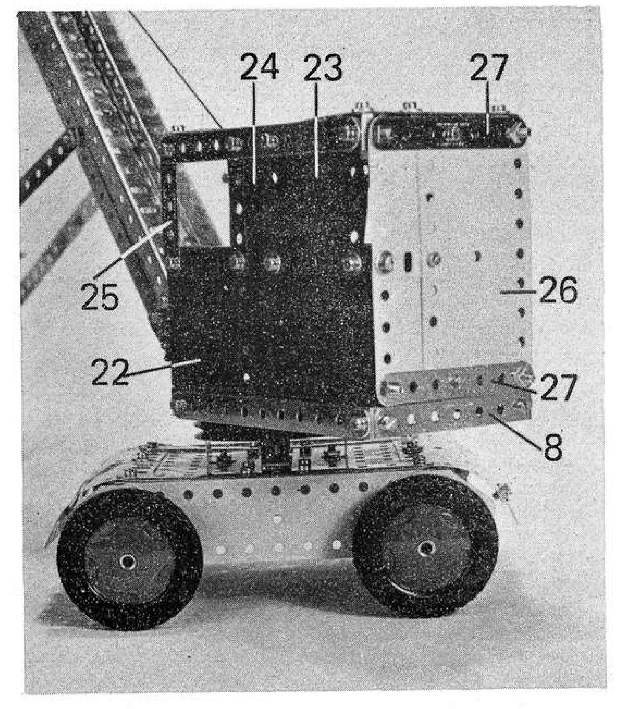
A close-up view of Mechanical Shovel showing the back and side of the body. The Bolts holding the back in place are first fixed Nuts in appropriate anchoring points, shanks pointing outwards, then the complete compound back plate is secured on the bolt shanks by further Nuts. This simplifies greatly what might otherwise be an awkward constructional problem.
