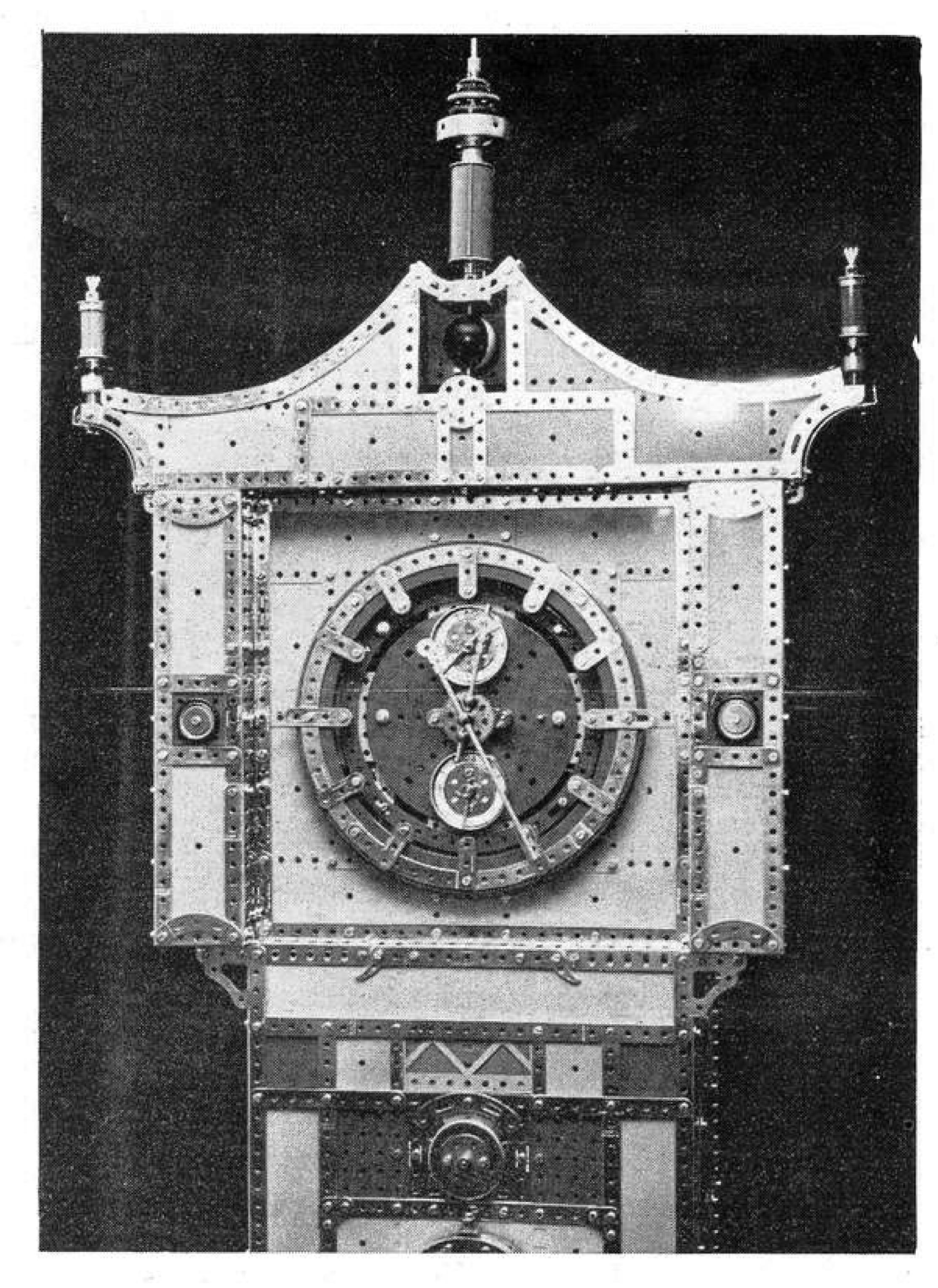
Opposite page: Fig. 1. General view of the No. 10 Set Grandfather Clock. The model stands 7ft. 4in. tall and runs for 26 hours on one winding. Above: Fig. 3. Front panel removed from clock-case to show pendulum and main driving weight. The pendulum has coarse and fine length adjustment. Fig. 4. View of ornamental top showing main and auxiliary dials with moon movement above. Upper small dial shows 24 hour motion. Right: Fig. 2. The clock base unit with lower end of the main clock-case showing
