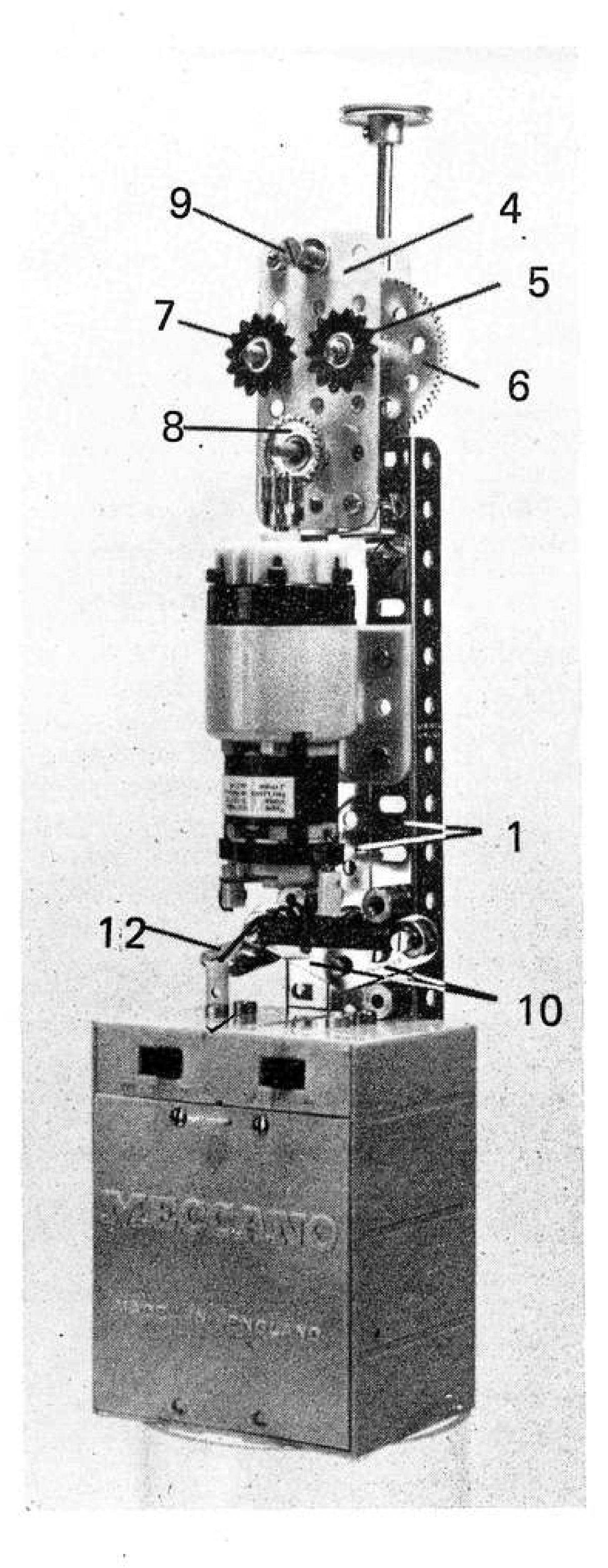
the Plate. A second 3½" x 1½" Flat Plate 4 is attached to the first Plate by a ½" Reversed Angle Bracket at the upper left-hand corner only, the lower corners being attached to Girders 1 by further Reversed Angle Brackets.
