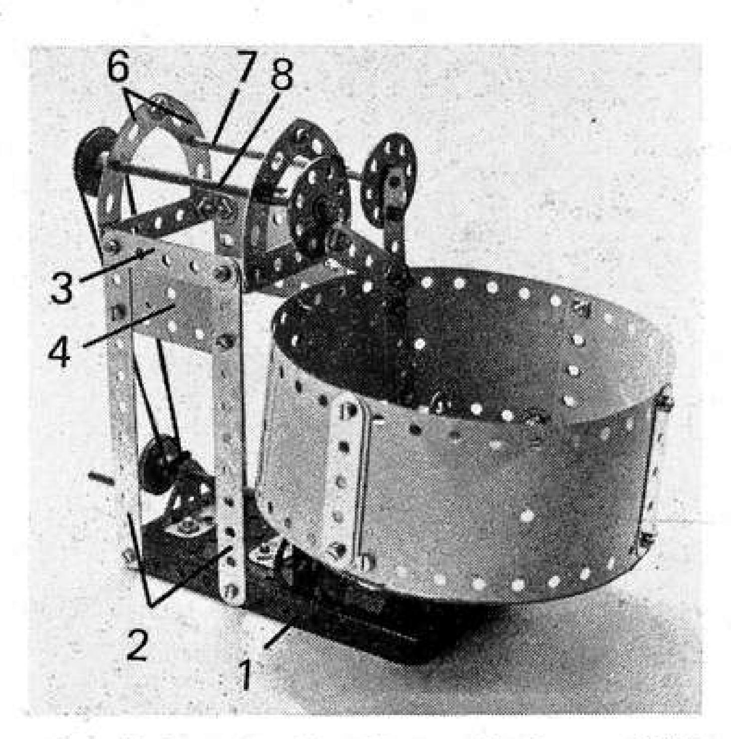
of which provide journals for a 3½" Crank Handle extended forward by a Rod Connector and a 1" Rod. The Crank Handle is held in place by the Rod Connector and by a Spring Clip and it carries in addition a 1" Pulley 13 which is connected to Pulley 9 by a 10" light Driving Band. Another 1" Pulley 14, fitted with a Rubber Ring, is fixed on the inner end of the 1" Rod.
