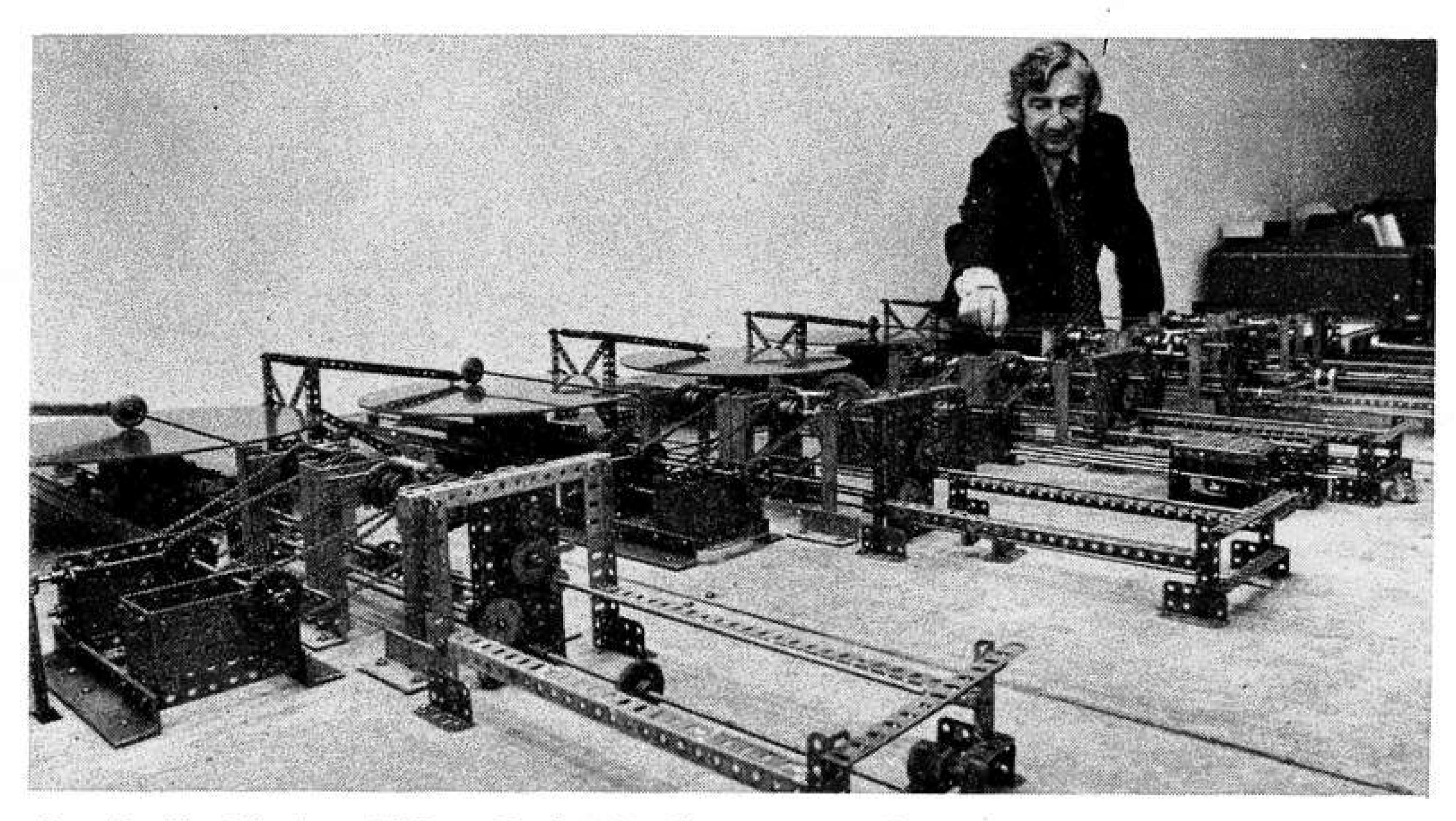
Dr. J. H. Whale of New Zealand adjusts part of a Meccano-built Differential Analyser — a type of computer — which was originally produced in England in the 1930's. Dr. Whale is restoring it to working condition for the Museum of Transport and Technology, Western Springs, New Zealand. (Photo reproduced by kind permission of the "New Zealand Herald".)
