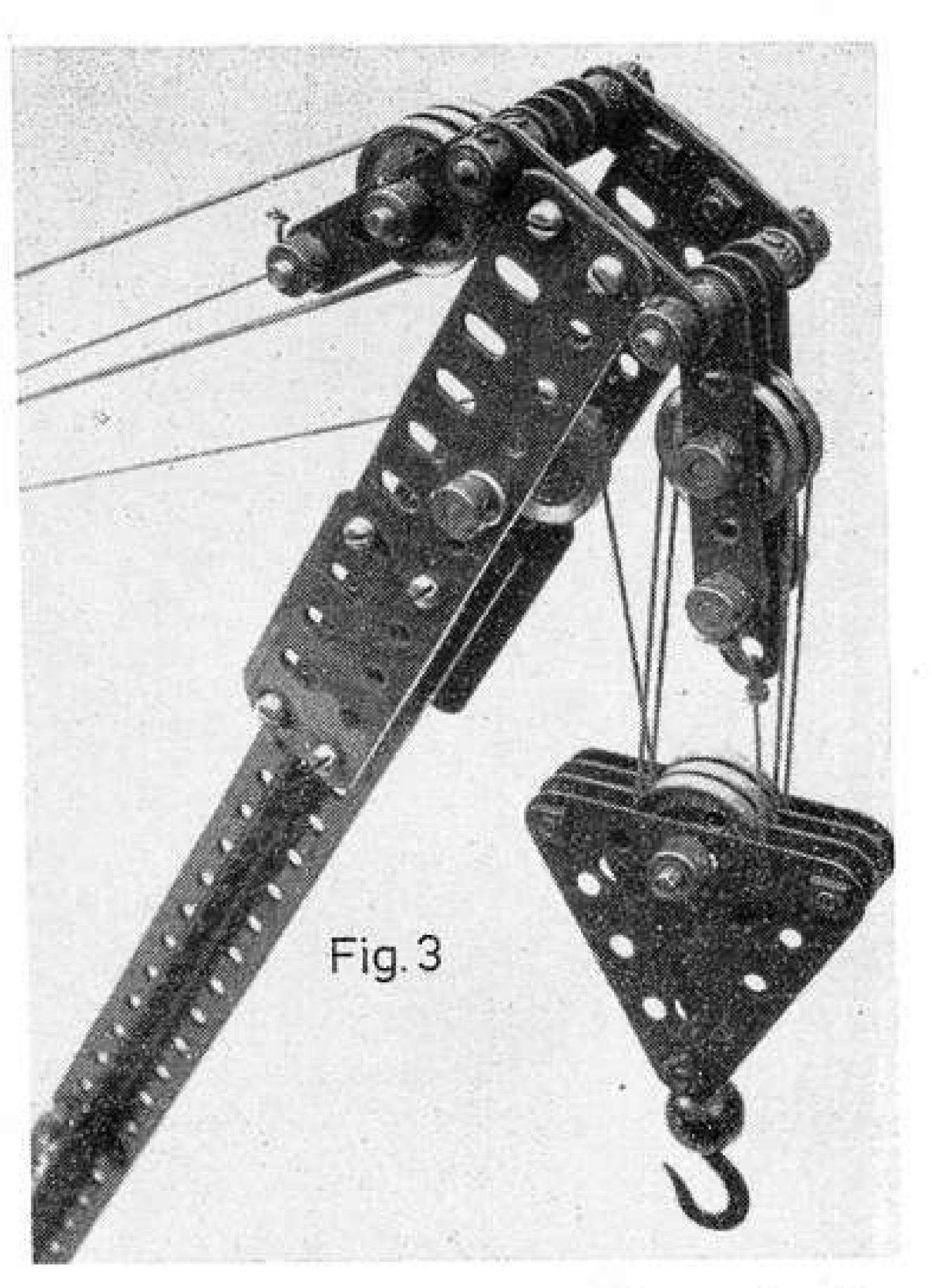
Close-up of jib head. Note double thickness of Flat Girders and 2" Strips to give a rigid structure.
