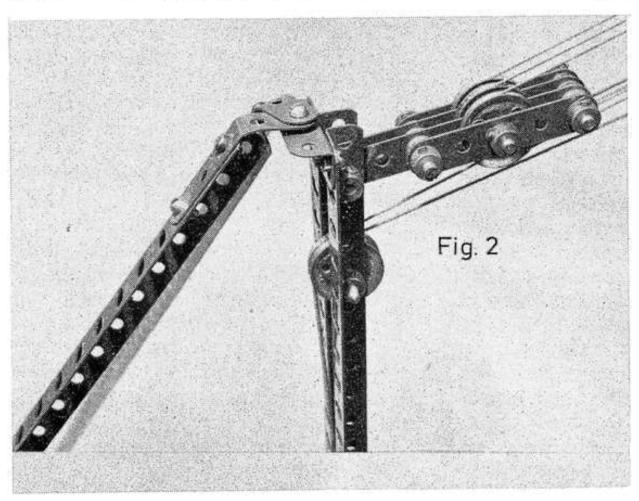
Opposite page, a general view of the "mystery" Super Model No. 6a — Steam-driven Stiff Leg Derrick, circa 1930. The jib radius indicator is a Standard Mechanism. Left, a close-up of the mast head pivot and luffing block.
