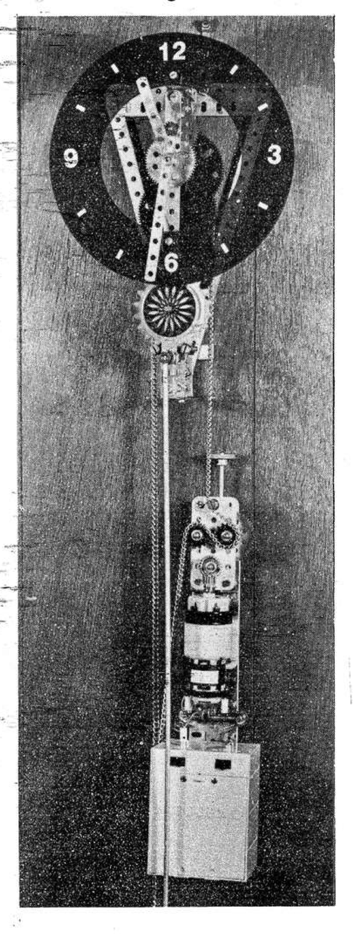
extended upwards by an 8" Rod fixed in a Rod Socket which is in turn secured to the spare lug of the 1" x ½" Angle Bracket bolted to the back of Strip 10. A 1" Pulley 13 is fixed on the upper end of the Rod, while a 7/16" Pinion is mounted on the output shaft of the motor, this meshing with Contrate Wheel 8. The motor gearbox is set in the 60:1 ratio.
