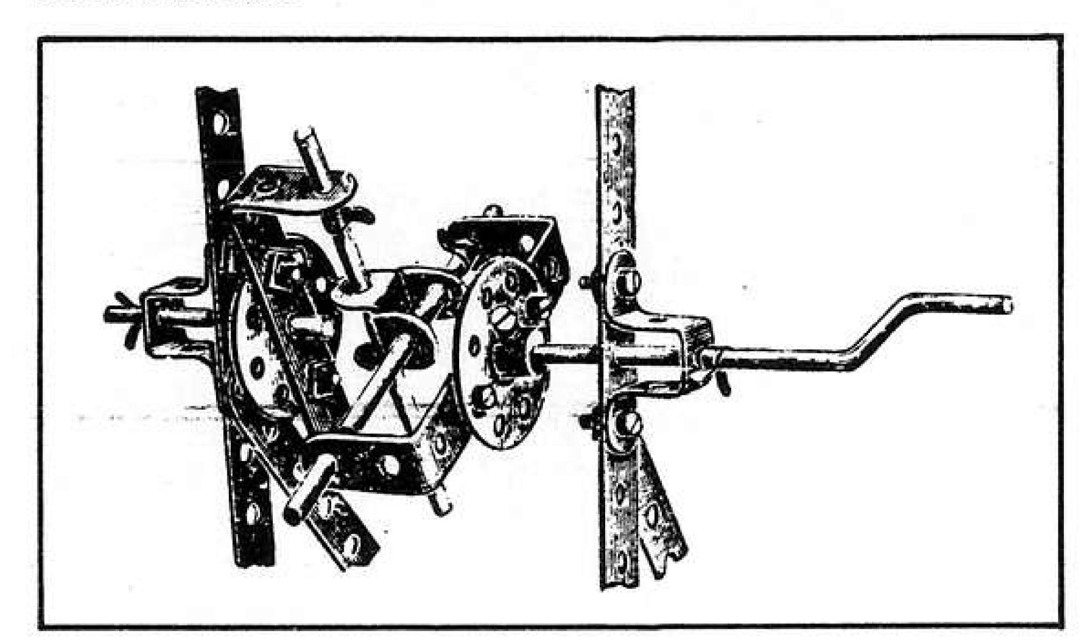
A sketch of a Meccano-built Hooke's Joint, reproduced from an early Meccano Manual. A clumsy affair compared with Part No. 140.
