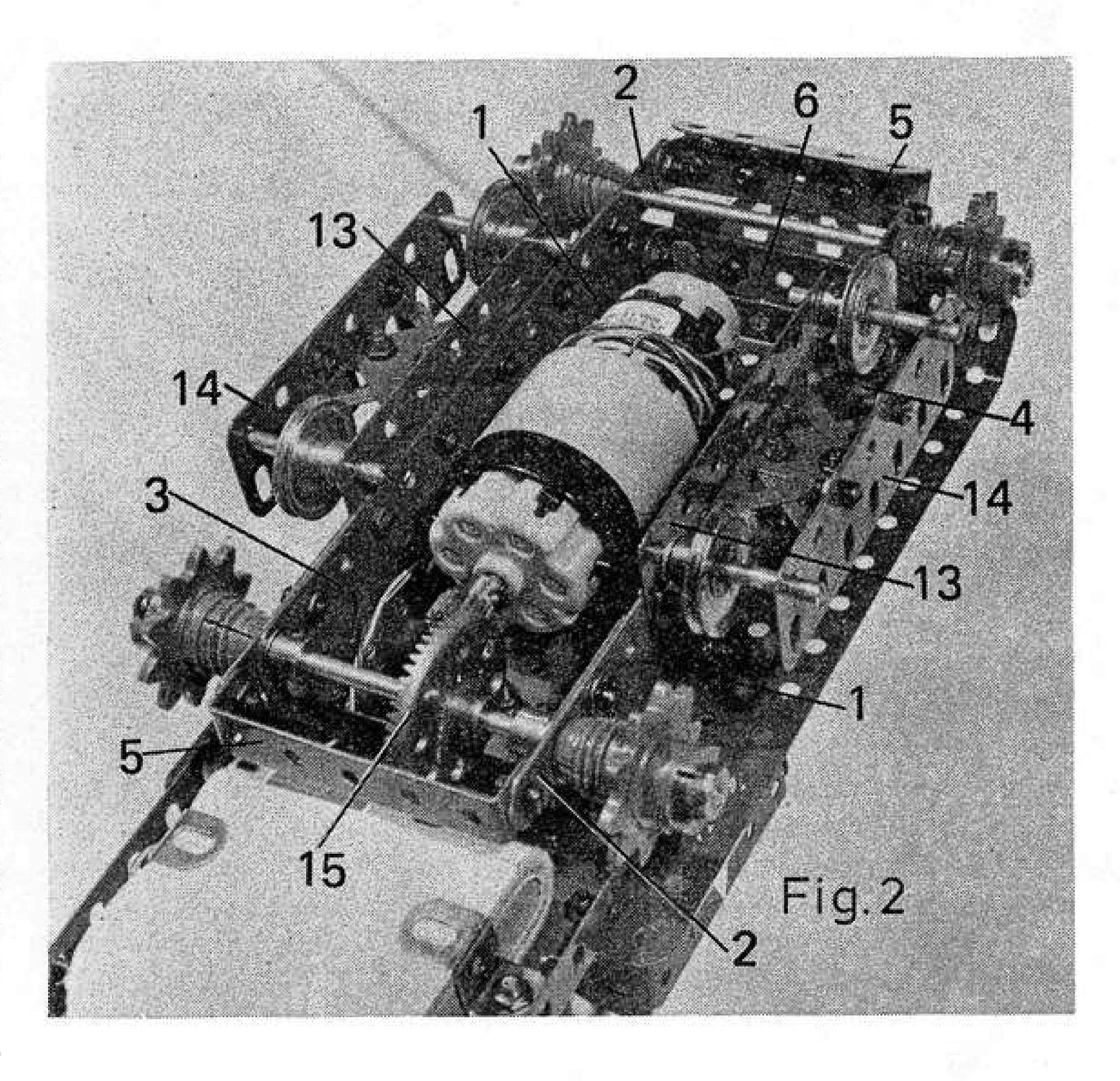
Manual. The unorthodox mounting of these latter Flat Trunnions gives a slope-front contour to the chassis plates at the front.
