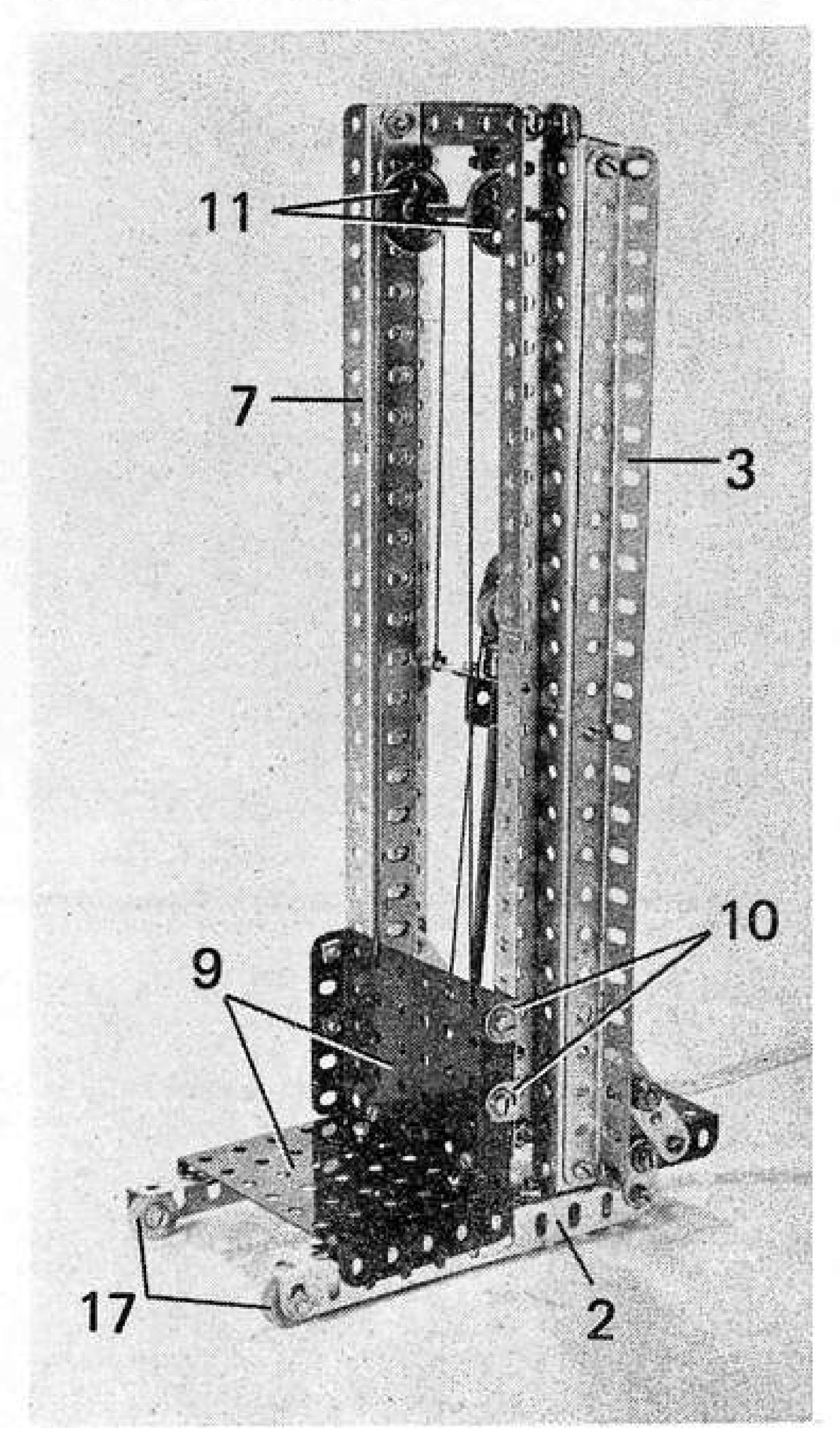
by Spring Clips. Revolving freely on this Rod are two 1" loose Pulleys 11 which are prevented from sliding on the Rod by further Spring Clips.
