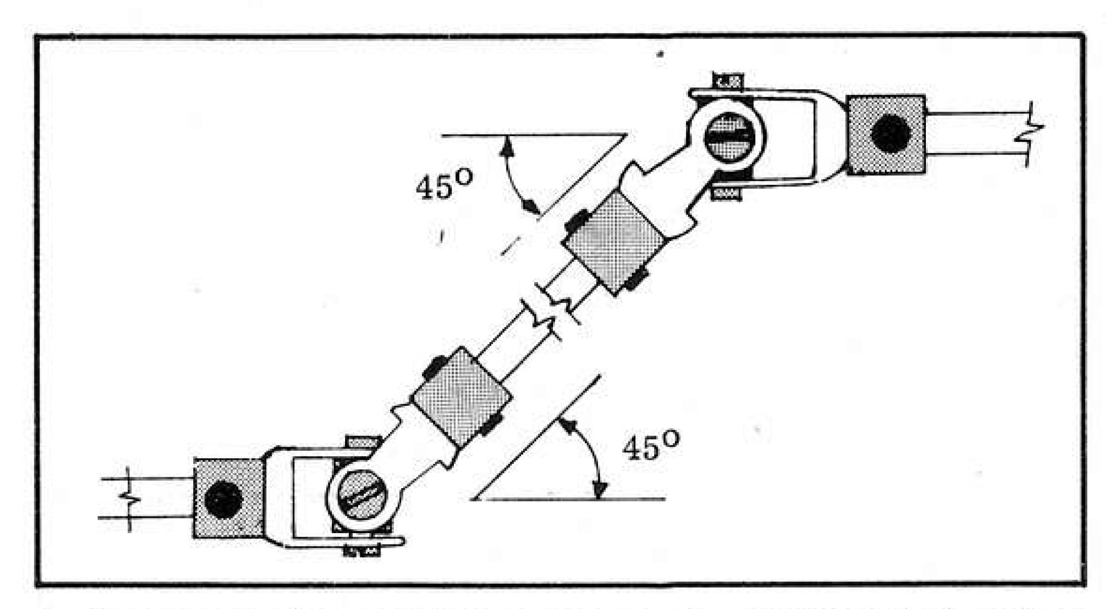
A sketch by the author showing the Universal Coupling arrangement which should be used to ensure that the driven shaft revolves at a constant speed. If a single Coupling is used, the speed of the driven shaft will vary.
