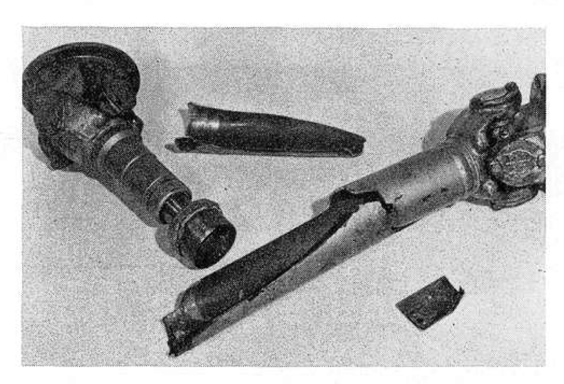
The dangers of ignoring engineering rules! A shattered full-size U.J. arrangement caused by spot-welding a balance weight (bottom right) to the intermediate shaft.
