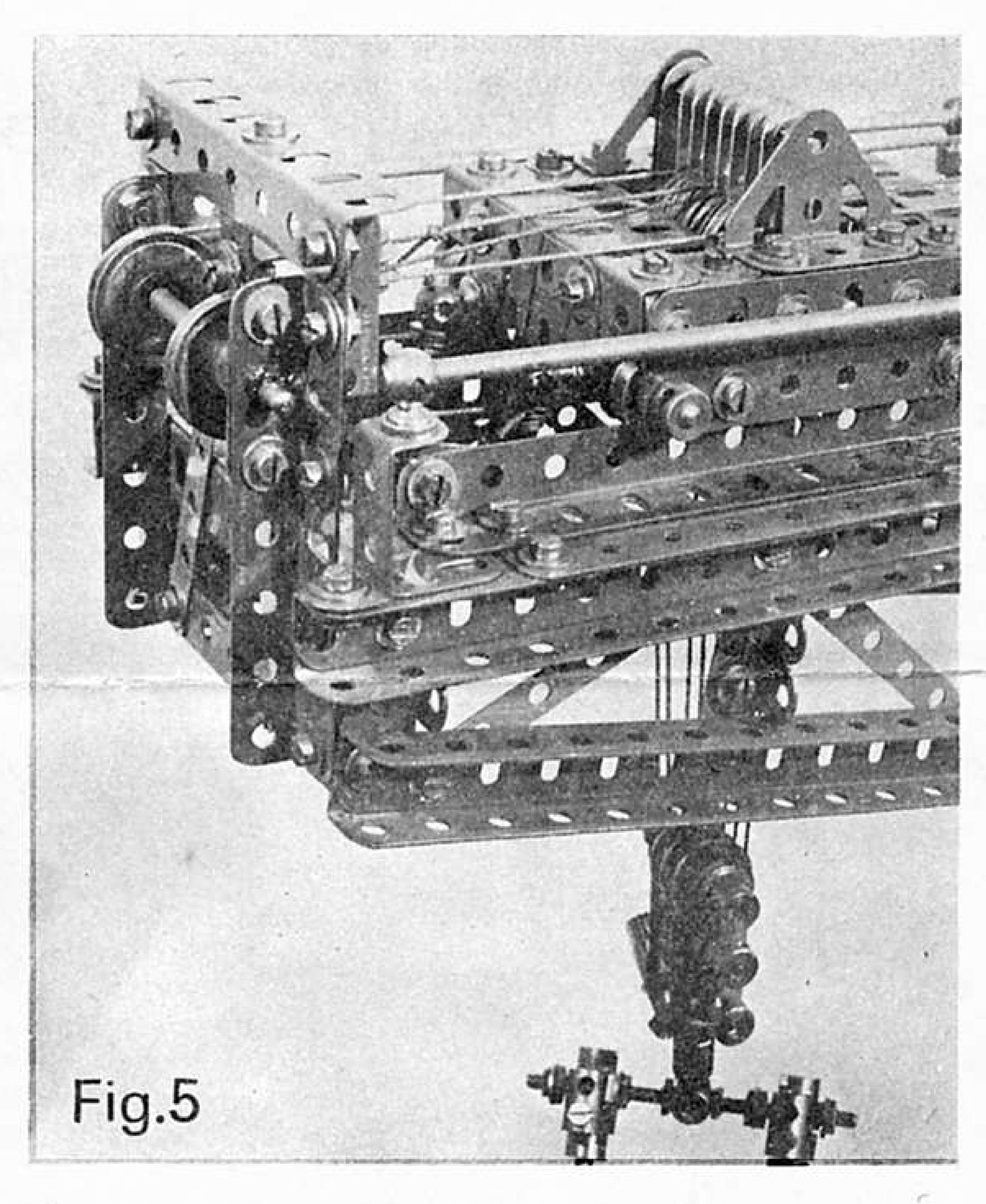
Two more photographs reproduced from the January 1975 MMQ. Left, the tower base showing details of final spur drive, ladderwork and auxiliary hook stowage. Right, gantry head details and trolley construction.
