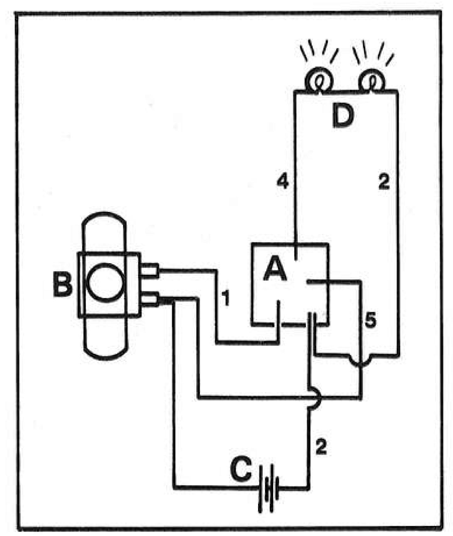
Wiring diagram showing method of using Electronic Control Set components for an Automatic Lighting System for a model car, suggested by Mr. Michael Walker of Darwen, Lancs A = Relay; B = Photo Cell; C = 12 volt D.C. power source; D = headlamps (a x 12v or 2 x 6v). Numbers indicate Relay sockets to which leads are connected.
