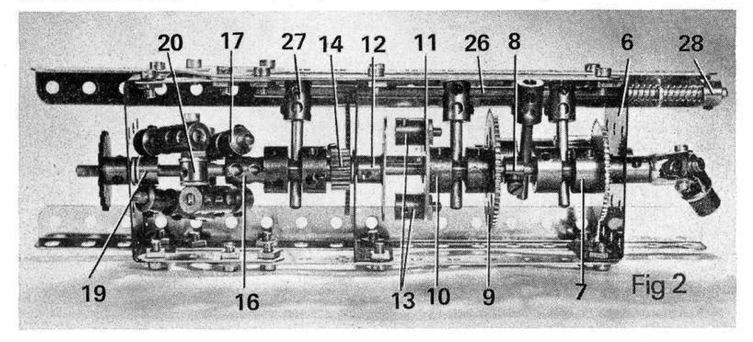
the permissible movement of the layshaft is governed by the fact that the Gear and Pinion must remain in mesh at all times. Fixed on the layshaft, between the Plates, is a ¾" x ½" Pinion 23, this being secured by a big 7/32" Grub Screw, This Screw locates (or not, as the case may be) with the slot in one end of a Socket Coupling 24, which is free to slide on the layshaft and in the other end of which a ½" Pinion 25 is fixed. This Pinion is also free to slide on the Rod.
