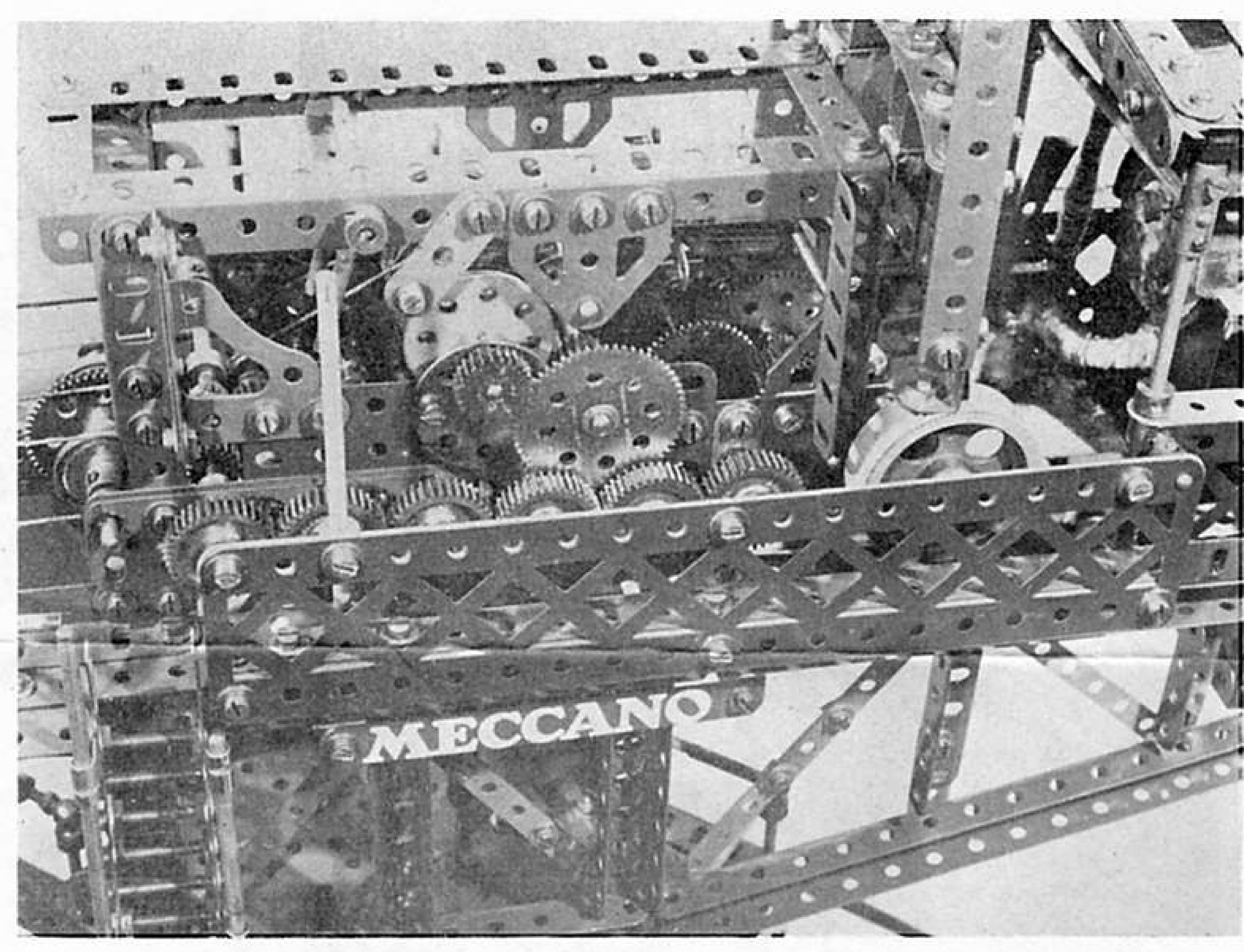
This photograph, reproduced from the January 1975 issue of the MMQ, shows the gearbox which is built into the Block-setting Crane. A diagramatical view of the gearbox, drawn by the author, appears below. A complex unit, it allows all movements of the model to be powered by one Meccano Steam Engine.
