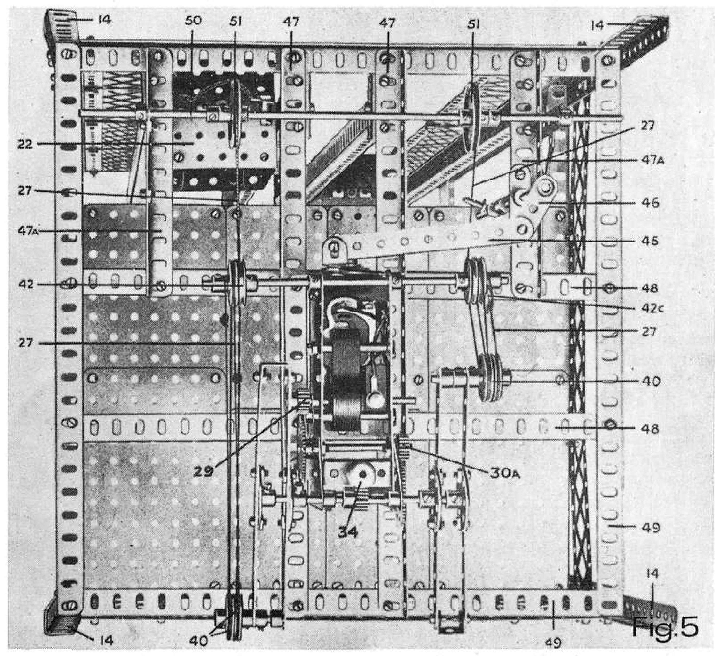
Fig.5, a plan view of the top floor of the Warehouse with the roof removed to show the arrangement of the Electrical Motor and the lift-drive mechanism. The motor illustrated is an obsolete 6 volt unit, but the current E15R Motor may be substituted with a simple modification.
