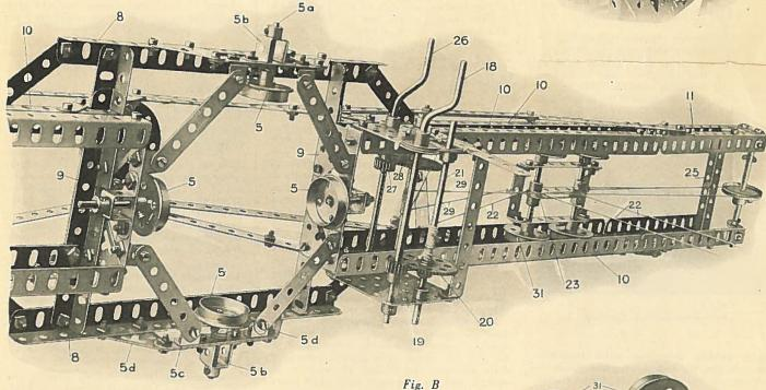
Radial cranes are used extensively in iron and steel yards and in lumber yards, where it is necessary to drop loads over a large area. The ground covered by the rotating cantilever arm is very considerable, and in some cases the arm is of great length. If it is desired to drop the load close in to the crane it is only necessary to run the travelling trolley (or truck) inwards along the arm. This enables the load to be dropped at any point between the base of the crane and the end of the arm.
