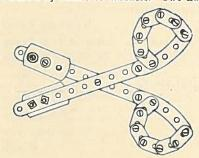
screwed to the bolts are used as a pivot and these are lock-nutted together by tightening one against the other, which prevents them from becoming loose. Enough play is allowed in the bolt to permit of easy movement of the strips. The following parts are required to build the scissors: 2 of No. 2, 2 of No. 90, 12 of No. 10, 4 of No. 38, 20 of No. 37, and 2 razor blades.
