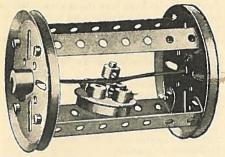
The weight illustrated comprises a Flanged Wheel carrying four Collars, the set-screws of which grip the shank of bolts passed
