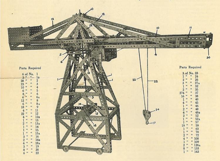
ing of the vertical rod 3 by which the cantilever arm 4 is turned.
