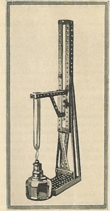
Test tube holder made from toy constructor parts, alcohol flame being used to heat contents of tube.
