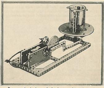
Rotary motion is given to beaker by motor-driven device shown.
