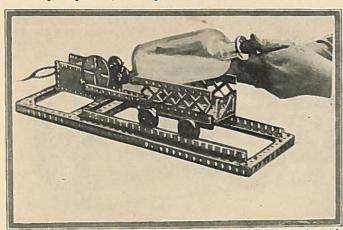
A very useful bottle churn which the amateur chemist can make with very little trouble from toy constructor parts, plus electric motor.
