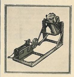
Photo above shows a test tube shaker comprising an oscillating carrier which is moved back and forth by crank connected to a disk on the electric motor.
