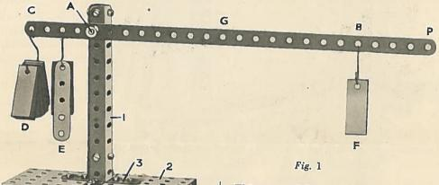
right member of this model is constructed from two 51/2" Angle Girders (1) secured to the base (2) by 1" x 1" Angle Brackets (3) and held together at their tops by two \\\'/2"x\\/2" Angle Brackets. A short Rod, which supports the lever, is passed through the upright and rigidly secured in a Crank bolted to the rear  $5\frac{1}{2}$  Angle Girder.
