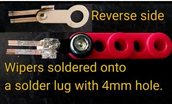
In the example above I have mounted the wiper onto a Meccano part number 260c Narrow Plastic Spacer but if you need the wiper to be orientated 90 degrees the solder lug can be bent around the 260c as shown in the example below.
