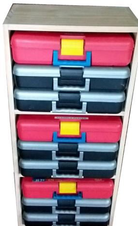
You will need 19mm thick dressed pine that is 275mm wide. These are standard sizes in Australia but near enough is good enough so long as each shelf is cut to exactly the same length. For this reason, you can specifically ask the timber store to use a jig to make sure each piece is cut to identical lengths. Measuring then cutting each shelf by sawing along pencil marks is doomed to fail. Most timber stores will cut to length and usually for free.
