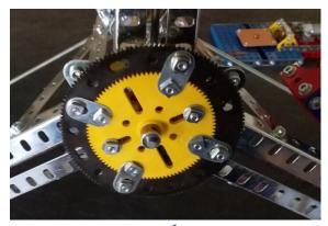
As the Cha Cha has 3 main radial arms a part 24b 6 Hole Bush Wheel was the obvious choice so I secured a triangle of 7 holes strips using Fishplates. My 1st thought was to use bevel gears but being rather rare and expensive I changed my mind and went for Contrates and pinions instead. Also the centre required 1 large Bevel and 3 small so that seemed a waste.
