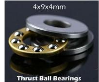
An interesting feature of these bearings is that only one of the ball races fits over a standard Meccano SWG8 rod which is 4.064mm. I tried them on a 4mm brass rod and one ball race was a tight fit while the other had quite a bit of movement.
