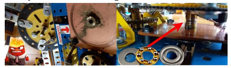
The weight of the Cha Cha was too much for the bosses even though they had 2 washers between ...use these 4mm thrust bearings
