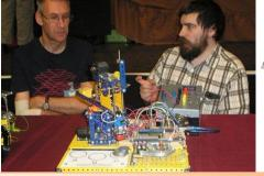
**Tower of Hanoi by Russ Carr** Another simple robot arm, but now with the Arduino programmed to solve the puzzle known as the Tower of Hanoi.
