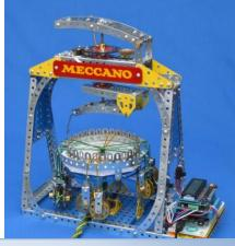
Kumihimo Braider by David Couch A hook, moved by a stepper motor and servo controlled by an Arduino lifts one thread at a time, moving it across the centre. The Arduino is programmed with 20 braiding patterns.
