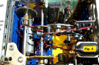
. The micro switch is mounted on a 12b Angle Bracket with a Fishplate to allow adjustment. It's better to use a micro switch with a long lever that extends past the body as this allows for more adjustment by bending the lever.
