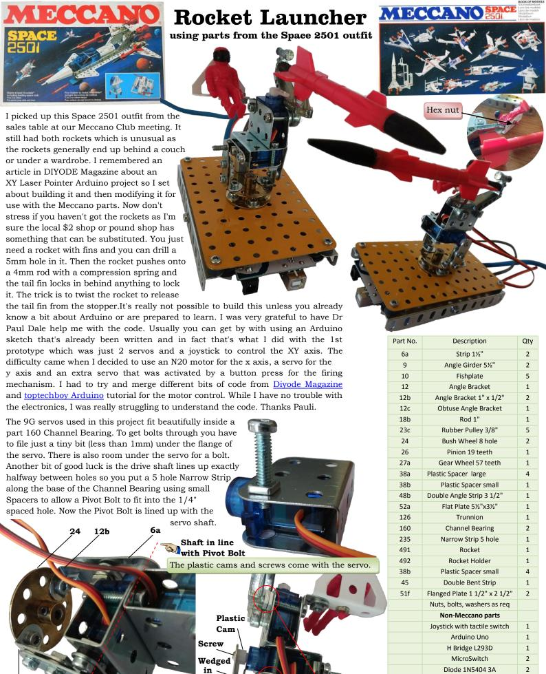
The Pivot Bolt is held in place by the 5 hole Narrow Strip.
