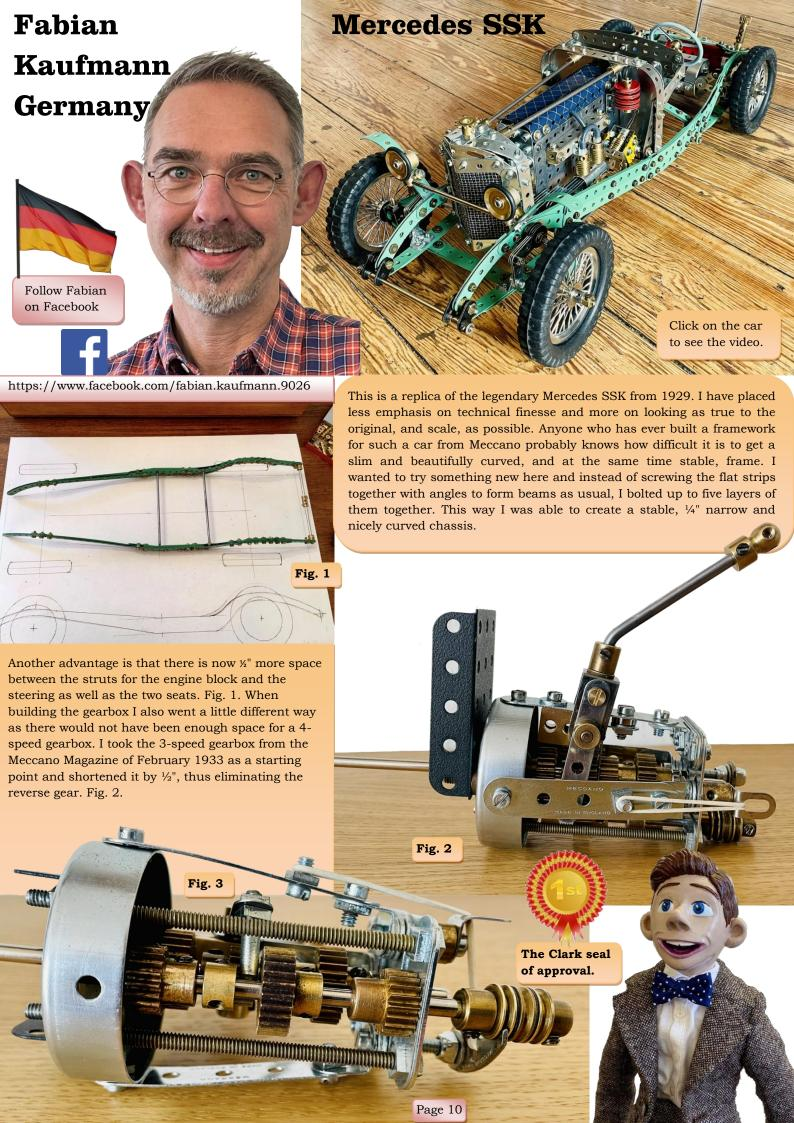
The gearbox is based on a non-standard pairing of 19t and 25t Pinions. Therefore it is difficult to connect it to other assemblies such as an engine block. To solve this problem, I moved the lay-shaft from its original position next to the main shaft downwards, so that the main shaft could sit centrally. Fig. 3. This way I could keep the original scale together with the engine block including the flanged steering gear. Fig. 4.
