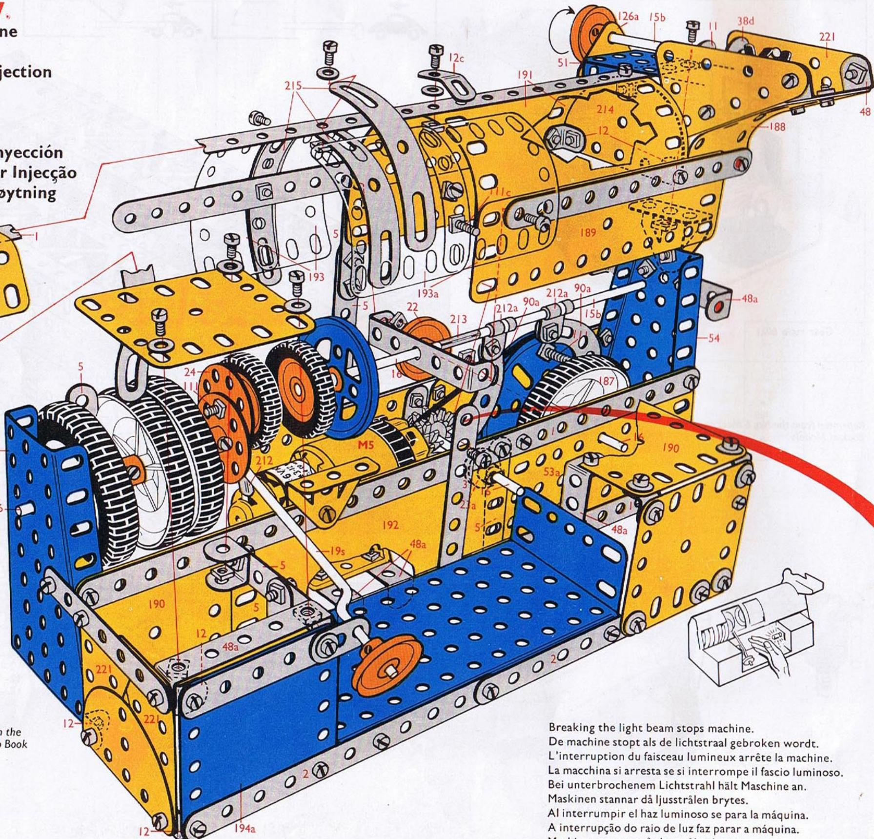
Breaking the light beam stops machine.
