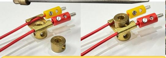
From Tim Gant – UK. A simple wire guide to keep things tidy. Just bolt it to the model any which way that suits. The collar traps the wires after they've been put in place. No need to thread anything through anything else - a process which can be very annoying.
