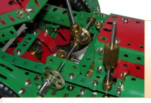
The instructions for the tipping mechanism are far from clear in French or English, and no illustration really shows it. I used a simple, manually operated, Threaded Rod mechanism, as a simulation for hydraulic lift.
