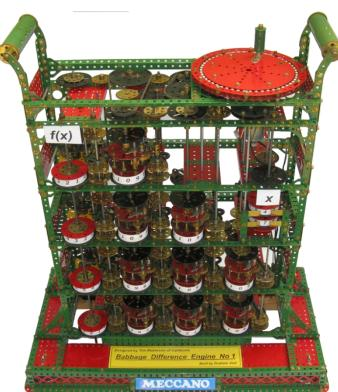
I added just two features to my build: a non-Meccano turntable for ready access to both sides, and an electric motor to drive it complete with dial indicating the current value of the variable. I found both features very useful.
