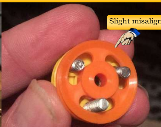
Bolt a part 22p Plastic Pulley with boss to 1" Plastic Pulleys without boss part 22bp.
