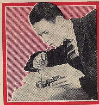
Fig. 4. A miniature smelting furnace formed by scraping a depression on a Charcoal Block.
