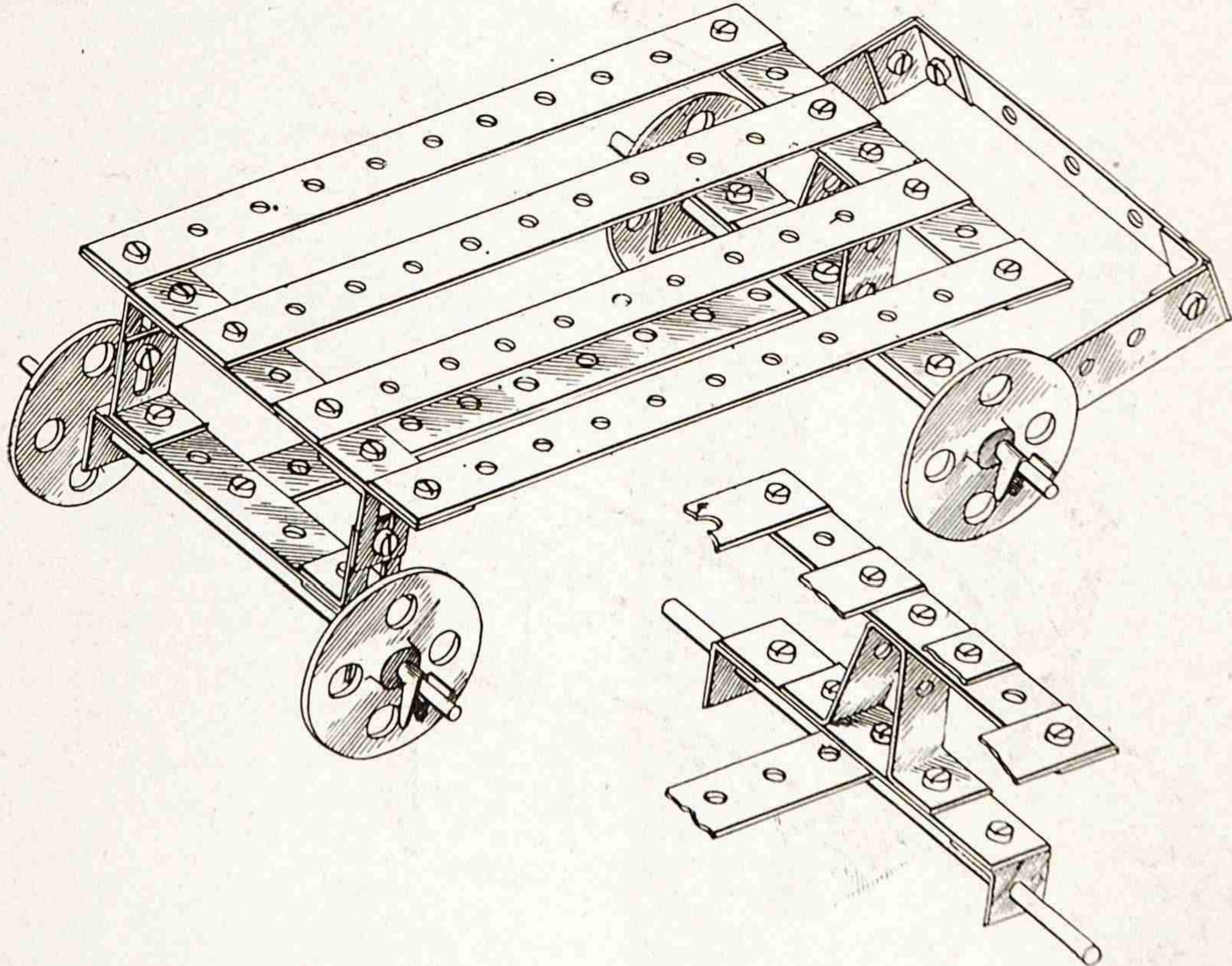
**Design No. 6. Tipping Waggon.**—The two end frames of this model are each built up of three  $2\frac{1}{2}$  in. strips. The bent piece at the back forms a stop for the waggon body to rest on. Pieces of cardboard, cut to size and shaped, are used to form the sides and bottom of the waggon, which swivels on the angle pieces about the centre holes of the nearest side strips.
