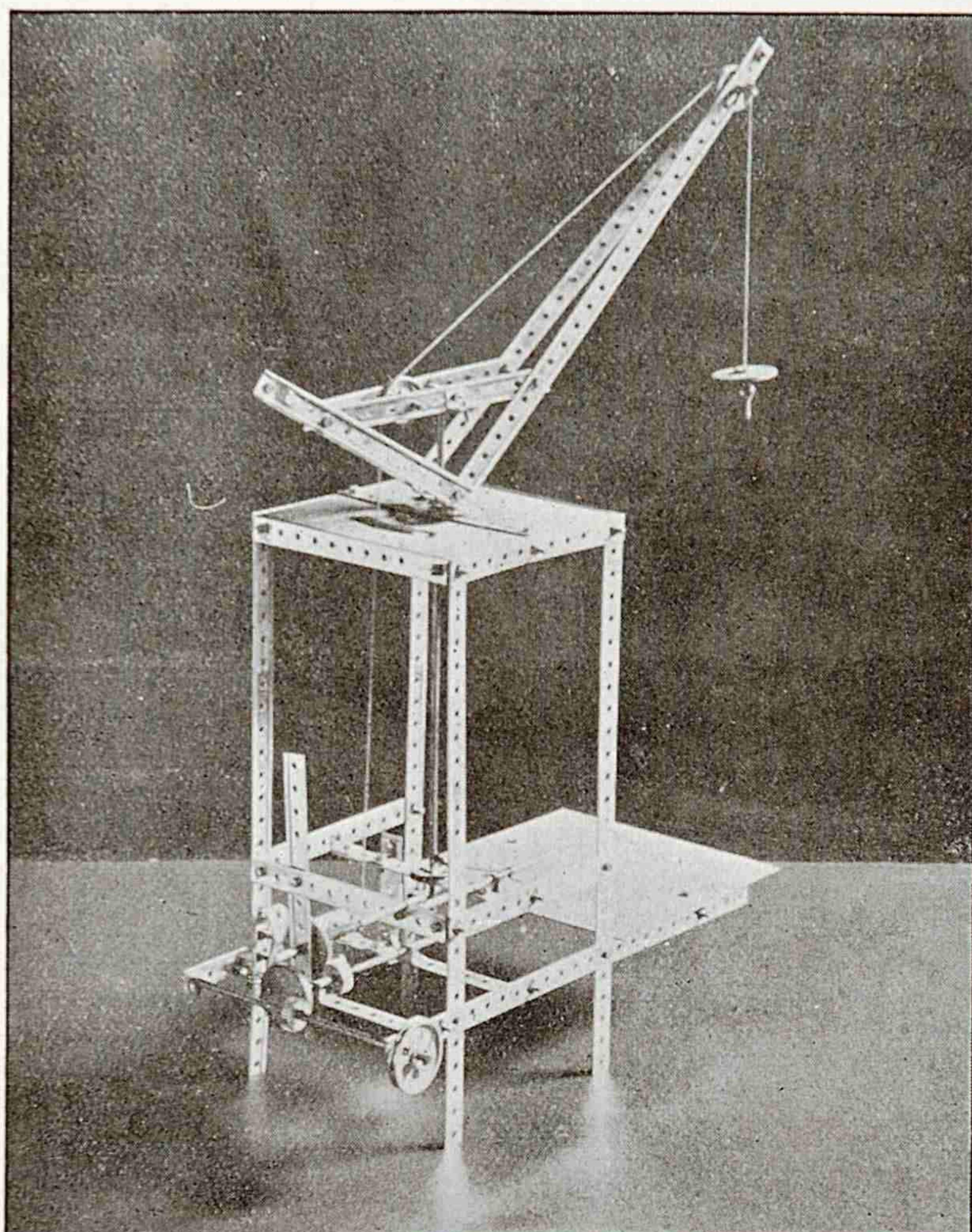
Design No. 14. Crane on Rails.—This model is made up in two distinct parts, separate views of which are given. The upper portion carries three cranked axles; the nearest one of these is for elevating or lowering the jib. The next horizontal one is for raising the load, while the upright crank is for rotating the whole upper structure of the crane. A gear wheel may just be seen in the sketch beneath the cross strip. When the upper structure is threaded over the upright
