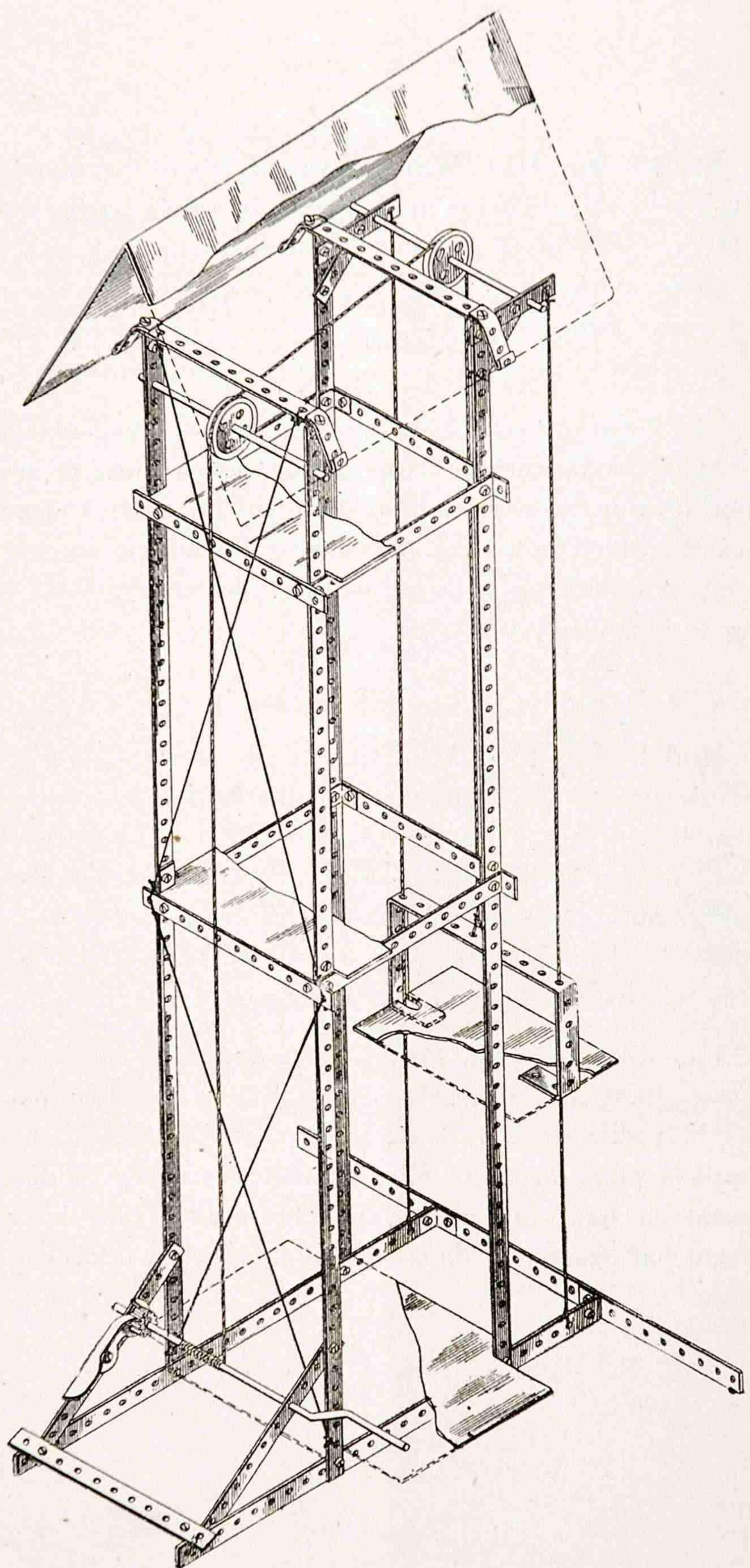
**Design No. 11. Cable Railway.**—The lines of rail in this model are constructed as in the first instance given. The outer wheel is where the driving power is received, and passing through the clutch mechanism, of which a separate detail is given, and the pair of gear wheels, it actuates the rope drive, which passes round pulleys at each end of the line of rails, one pulley being on the same axle as the gear wheel.
