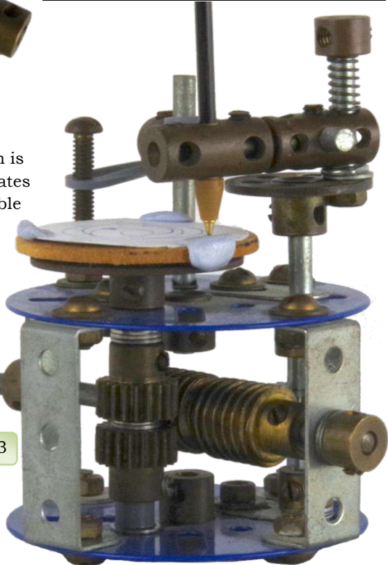
Fig. 2. The driving Crank Handle is journaled in the central hole of a pair of Double Angle Strips as illustrated. The Crank Handle has two Worms attached. One drives a 25t Pinion, the other a pair of 1/2" Pinions, one having 19 teeth and the 2nd (green) being the obsolete 20t version.
