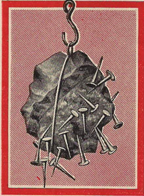
Fig. 1. Lodestone that has been dipped in a heap of tacks.
